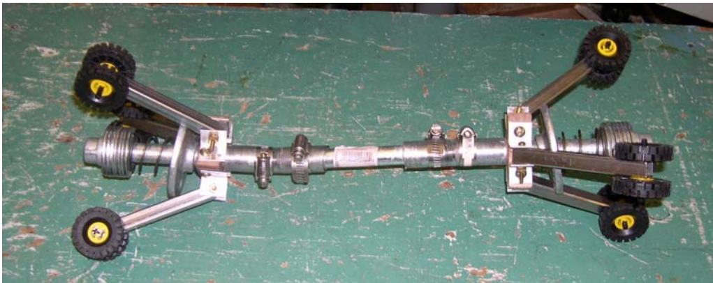
Fig. 2-1. Early attempt at guide wheels using angled wheel mounts actuated by one large compression spring.
